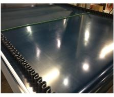
Belts can be made out of PVC or Urethane to handle different levels of abrasion
